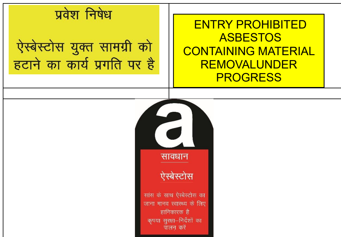
Fig.No.2 Asbestos warning signage
