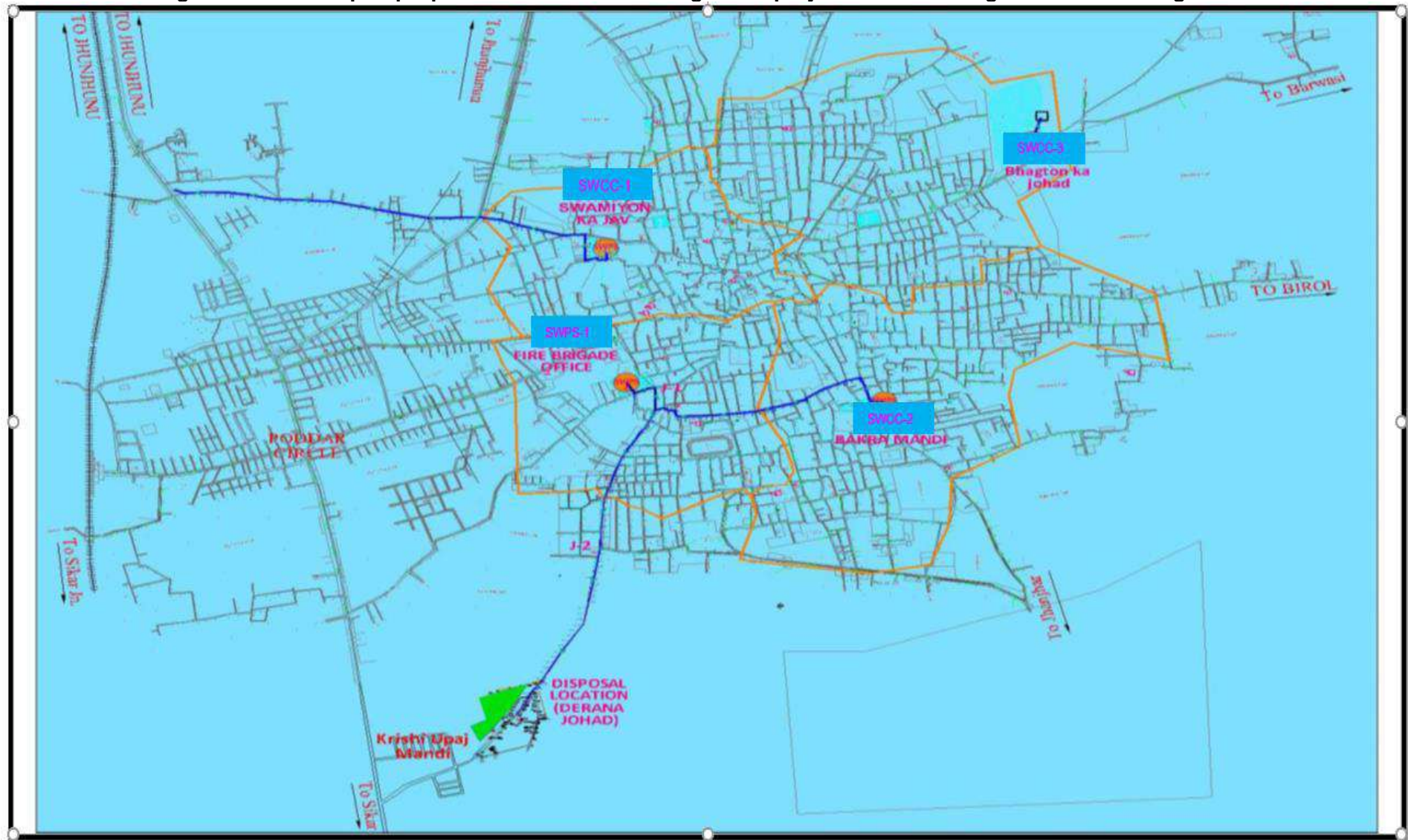
Figure 3: Index map of proposed Storm water management project work showing SWPS and Rising Mains.
