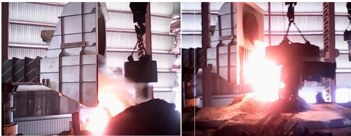
Figure 5. 9: Working of side-based Suction Hood
